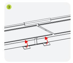
Fold the two tabs on the lower edge of the joint to fix it.
