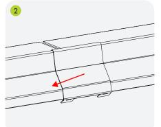
Overlap the joint with the profiles to hide the gap between them.
