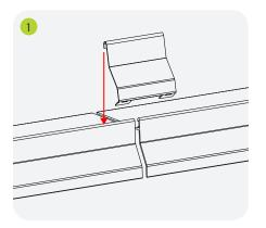
Place the upper side of the joint on the outer edge of the two profiles placed side by side.
